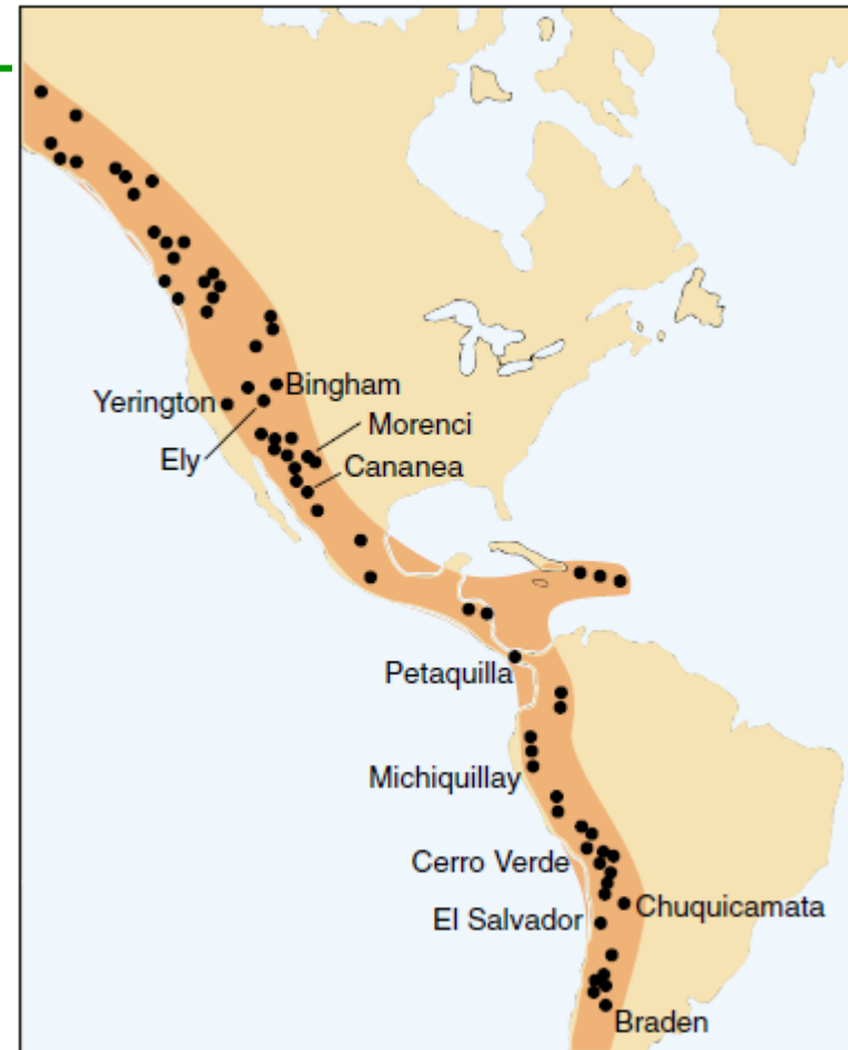
Figure. Porphyry copper deposits in the Western Hemisphere lie along modern or ancient tectonic plate boundaries.
