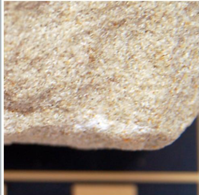
CLASTIC TEXTURE Visible grains, sand-size; the rock feels gritty to the touch (grain size between 1/16 and 2 mm)
